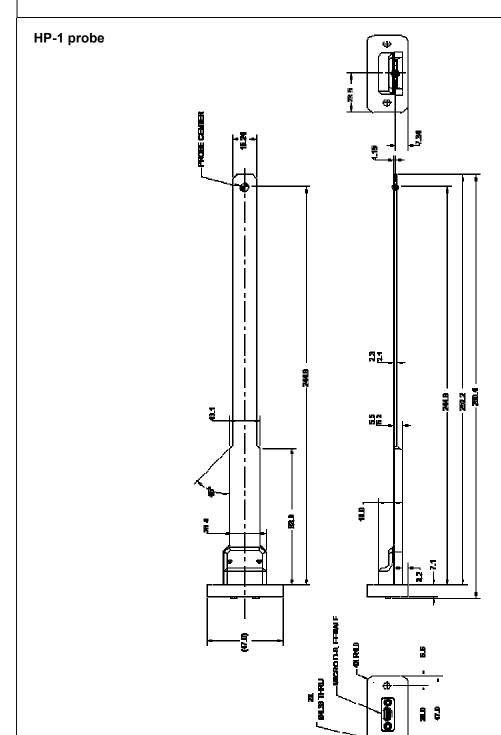
Positive (N to S) field vector into probe axis marker gives positive field reading
