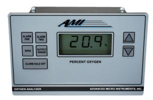
The AMI model 70R1 is the ideal solution for measuring oxygen in non-flammable gases in a general purpose environment. In a very small size, and at low cost, it provides a complete electronic package with a full set of features together with a zirconium oxide sensor that has an expected ten year life, with virtually no calibration required.
