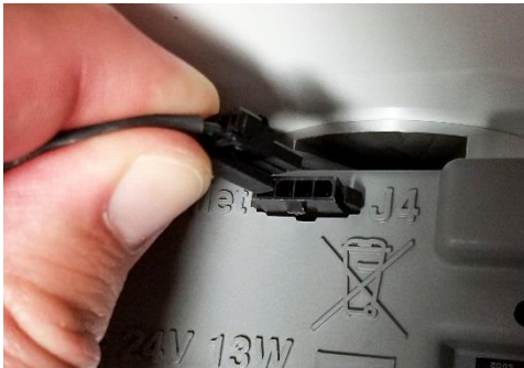
Figure 19: Disconnect heated inlet cable
