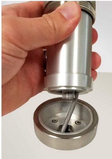
Figure 21: Pull heated inlet assembly up
