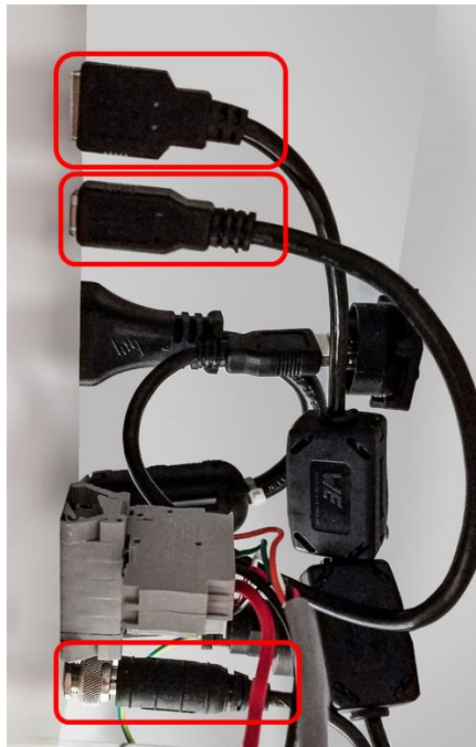
Figure 23: Removing USB and power cables
