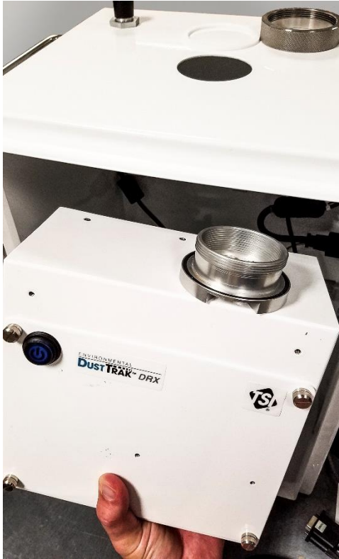
Figure 28: Removing the instrument from enclosure
