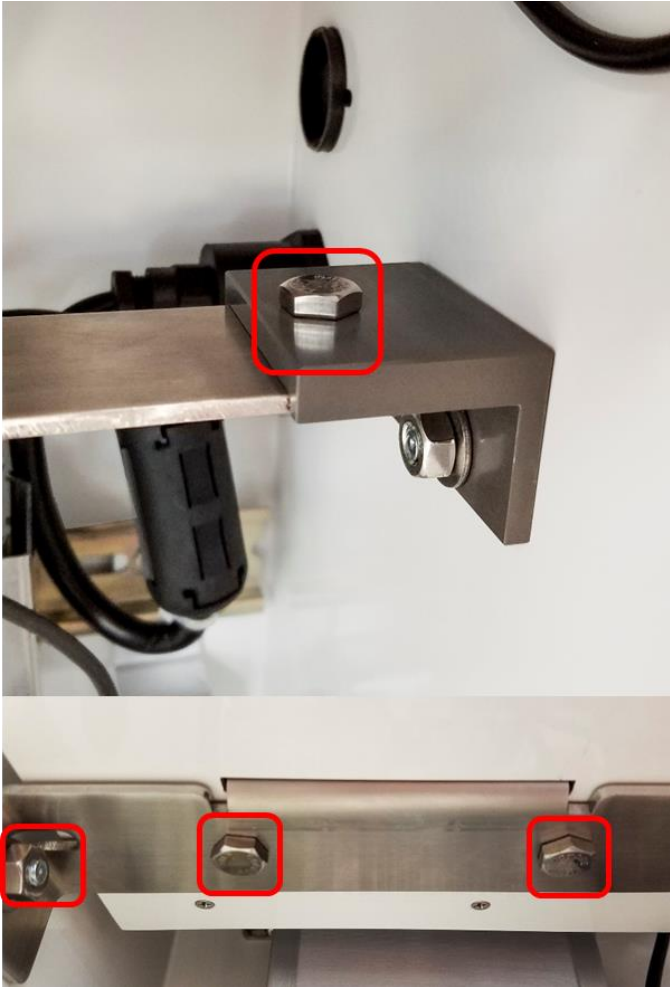
Figure 26: Removing instrument from mounting bracket
