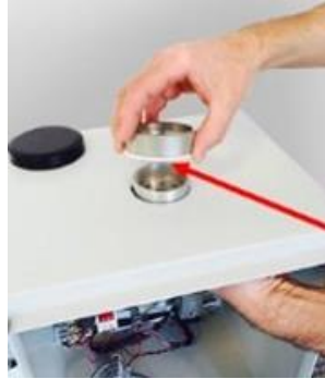
Figure 35: Secure retainer ring
