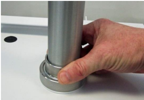
Figure 38: Secure inlet column to retainer ring
