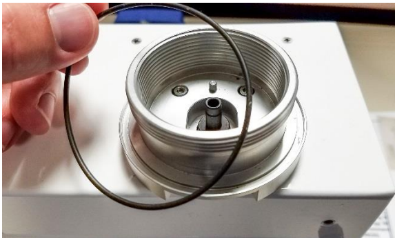
Figure 29: Removing rubber O-ring from mounting ring
