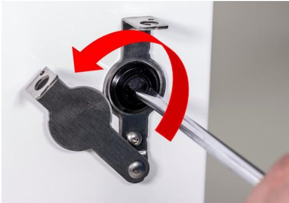
Figure 3: Opening the enclosure
