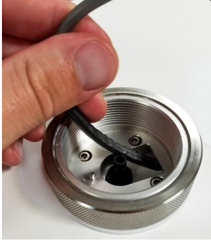
Figure 22: Removing heated inlet assembly
