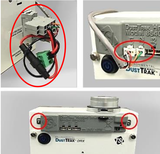
Figure 30: Removing cables and heated inlet controller
