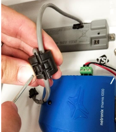
Figure 20: Removing ferrite clamp assembly
