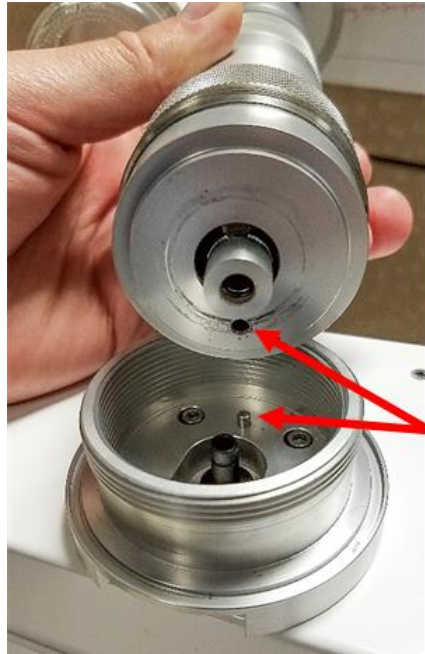
Figure 37: Aligning inlet assembly
