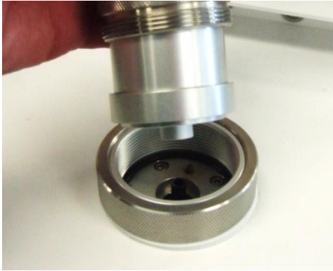
Figure 18: Remove inlet assembly
