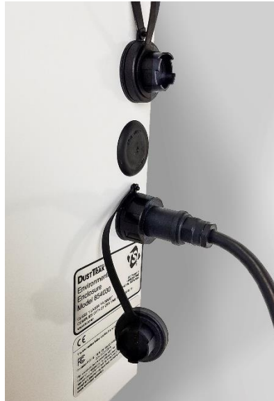
Figure 8: Connecting power cord
