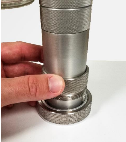
Figure 17: Unscrew the top knurled ring
