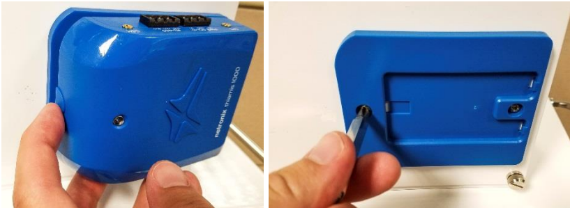
Figure 31: Removing Thiamis™ 1000 modem
