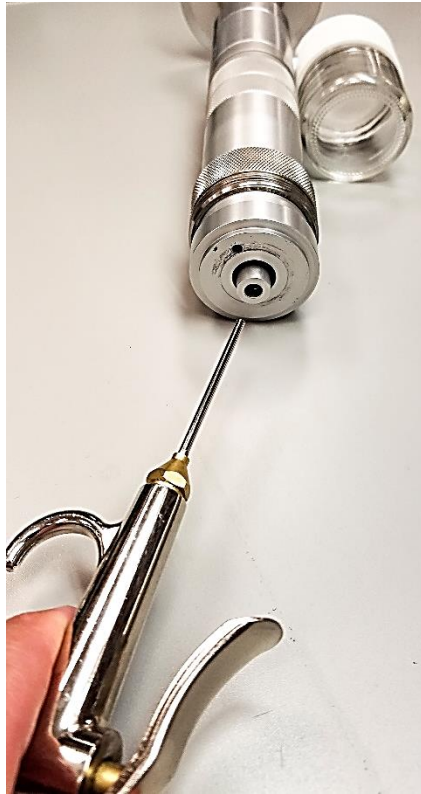
Figure 39: Blowing compressed air through the inlet
