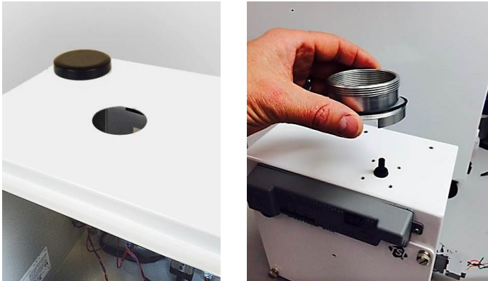
Figure 34: Remove mounting ring from photometer
