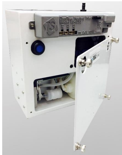
Figure 26: Open instrument service panel
