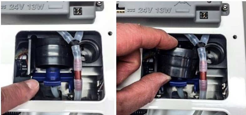
Figure 33: Release and remove cassette holder
