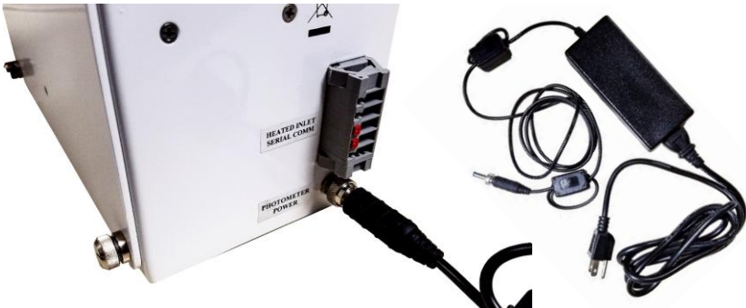
Figure 5: Instrument power connection
