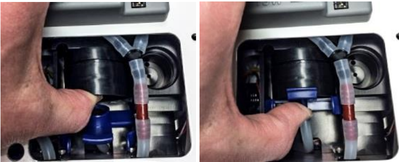
Figure 35: Snap cassette securely into inlet port
