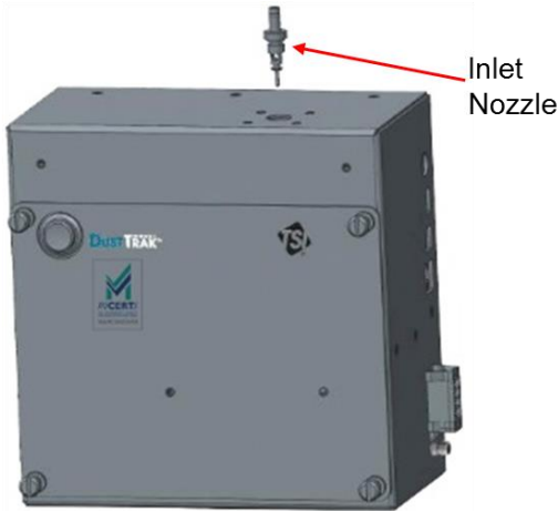
Figure 17: Unscrew Inlet Nozzle
