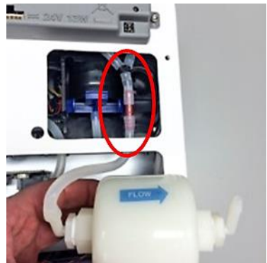
Figure 22: Replace with new filter
