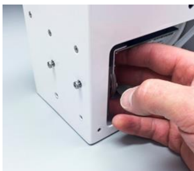
Figure 31: Secure new pump
