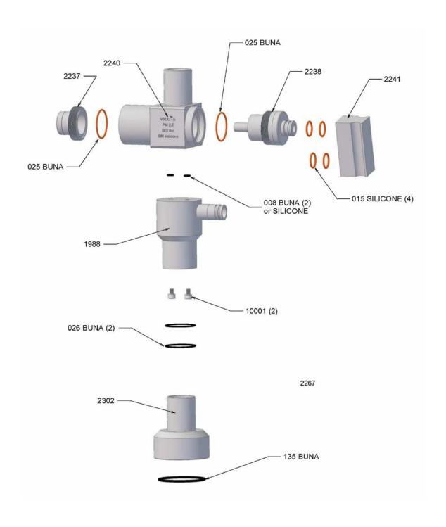
Figure 4c: Exploded view of VSCCA® Showing 2302 Outlet Adaptor for Graseby/Anderson RAAS™ System
