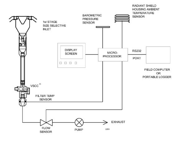
Figure 2: Generic FRM Sampler Showing VSCC® Installed
