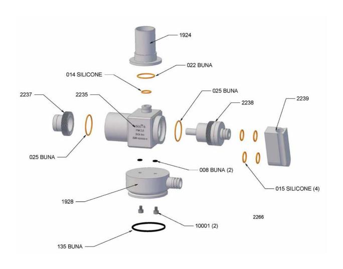
Figure 4b: Exploded View of VSCCB®
