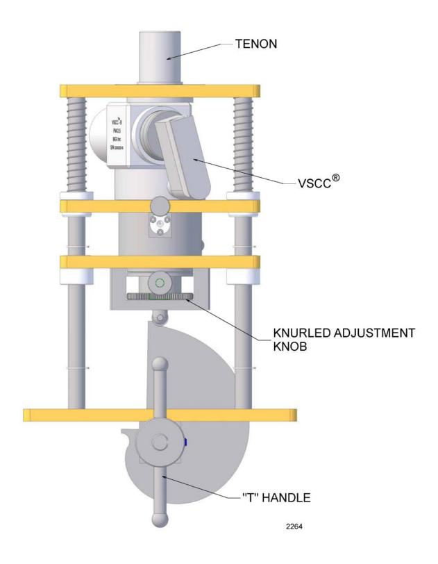
Figure 3: Drawing of VSCCB® Installed in the BGI PQ200 or PQ200A
