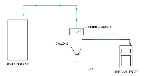
Schematic Diagram of Connections for Calibrating a Personal Sampling Cyclone
