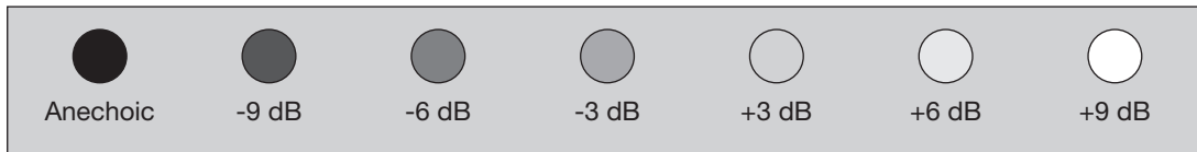
Test objects have same speed and attenuation as background
