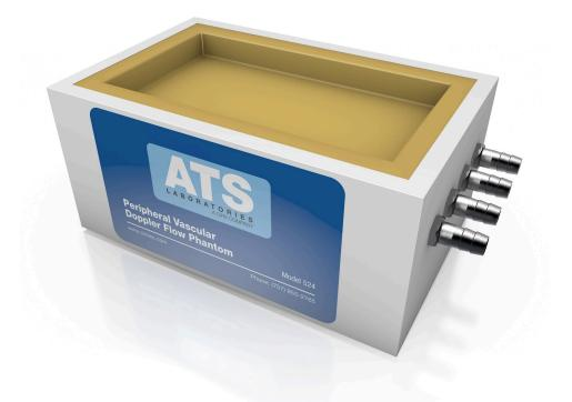
The Models 524 and 525 tissue mimicking Doppler flow phantoms contain four flow channels simulating superficial vasculature. The simulated vessels are located 15 mm below the scan surface. Built-in scanning wells are provided to permit the use of water or a low viscosity gel as acoustic coupling agents.
