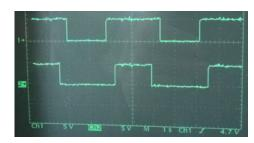
Square-waves of the target motion position as seen on an oscilloscope
