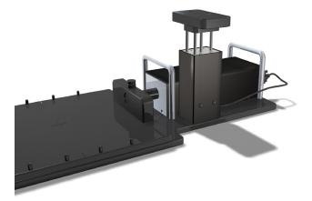
The surrogate motion is mechanically independent of platform motion and programmable through the CIRS Motion Control Software. This feature provides even greater flexibility to the clinician and is useful in assessing correlation between surrogate and phantom motion.
