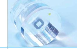
The QUART DVTap phantom is designed to be used as a technical tool for QA/QC testing in Cone Beam CT (CBCT), Dental Volume Tomography (DVT) and 3D Imaging applications.
